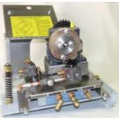
The Bear Cat Twin-Stop is the premier safety device that sets the brake to stop the drawworks motion in both directions. It engages the drawwork's brake automatically, in
